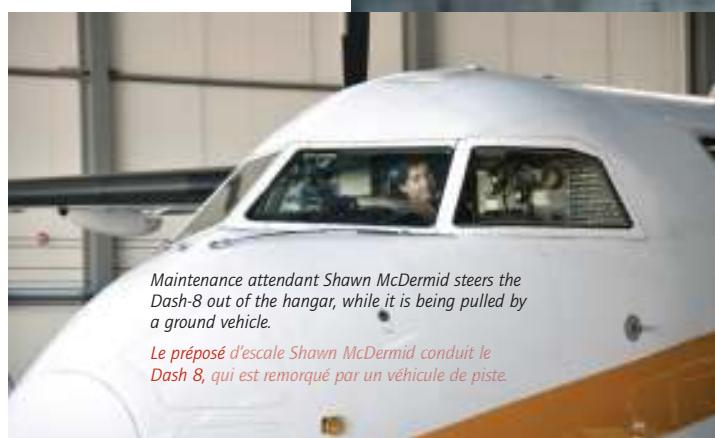
*Maintenance attendant Shawn McDermid steers the Dash-8 out of the hangar, while it is being pulled by a ground vehicle.*
